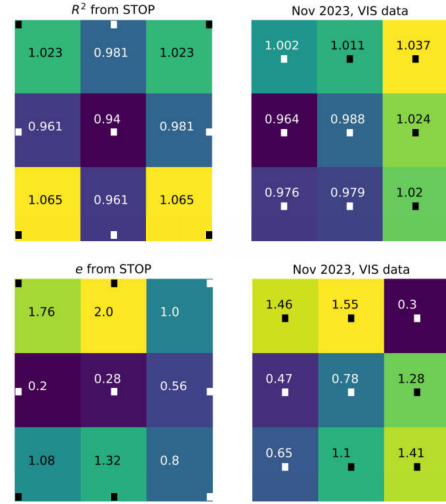
Fig. 9. Visualisation of the relative variation of R^2 and e over the VIS focal plane, +X to the right and +Y going up. The values have been normalised by the average of the nine values, with an average R^2 of 0.0479 and 0.0199 \text{ arcsec}^2 and an average e of 0.025 and 0.021 for the STOP and in-orbit data, respectively. The difference between the values are due to the use of a different Gaussian weighting in the calculation of the moments (see Sect. 5.3.2). The squares mark the reference positions on the FPA where the values have been obtained. Left diagrams: relative R^2 (top) and e (bottom) predicted by the STOP analysis. Right diagrams: relative R^2 and e measured in orbit in November 2023.
